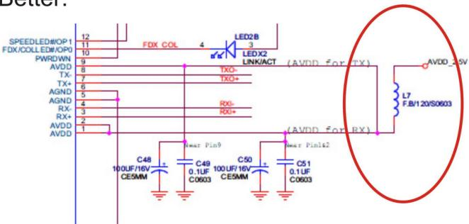
In this configuration the high frequency components can be filtered by the bead. The top circuit cannot filter them, because Pin 9 provides a low impedance for them to pass through.
