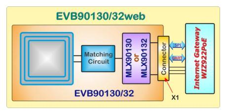
The RFID/NFC Reader Board is a universal HF frontend for mobile and stationary 13.56MHz reading devices. The MLX90130 or MLX90132 RFID-Transceiver IC from Melexis used here supports all commonly used standards like:
