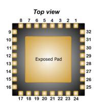
The device is packaged in a 32 pin lead free QFN package
